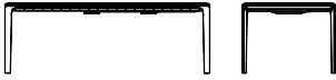
INVITO extension table / Auszugstisch H 76 W 1200 + 1x450 W 1400 + 1x550 W 1600 + 1x550 W 1600 + 2x400 W 1800 + 2x500 W 2000 + 2x550 W 2200 + 2x550 D 104, 94 CM
